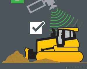
Dealer views engine-misfire reading via remote diagnostics connection and matches symptoms with a service bulletin identifying an update. Dealer deploys an Electronic Control Unit (ECU) payload via remote programming to update software and resolve problem.
